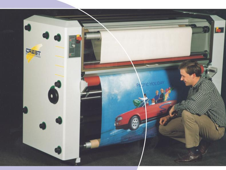
This 167 cm roll-feed hot/cold transfer laminator can be partnered with any digital toner printer. Using heat and pressure the laminator transfers the print's toner layer to self-adhesive marking films. The 1600 TTL will also apply overlaminates (clears) 'in line'.
